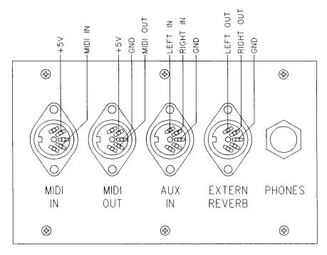
The external connections @ (several DIN connectors) and the headphones socket can be found on the left side beneath the keyboard shelf (see above drawing). The functions of these connectors are the following:
